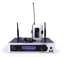
The S5.3-L includes a beltpack transmitter with a lavalier microphone and a true diversity tuner. Both of them feature user-friendly operability, and employ an easy-to-read LCD display. Also it is possible to perform the system settings through infrared communications, and monitor the system status using the supplied PC software.
