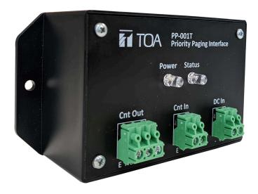
The PP-001T is a Priority Paging Interface that connects TOA's 9000 series Modular Digital Matrix Mixer/Amplifiers to TOA's M-864D Digital Stereo Mixer, to add paging functions with priority to the M-864D. The PP-001T can connect to any third party mixer or amplifier that can provide Dry Contact Output.
