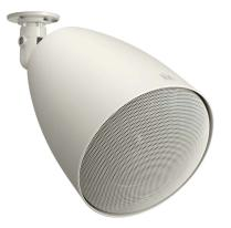
The PJ-64 is a projection speaker designed for ceiling and wall installations. Considered in architectural design, it can blend in with lighting equipment. The supplied swivel bracket allows for flexible speaker angle adjustment. The PJ-64 is driven on high-impedance (100 V and 70 V) line. The input power (impedance) can be easily changed at the upper side of the speaker. The speaker is easy to repaint so as to meet a wide range of design needs.
