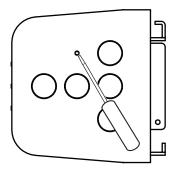
**Step 2.** Hold down the Mute switch while confirming that the Power indicator lights blue.
