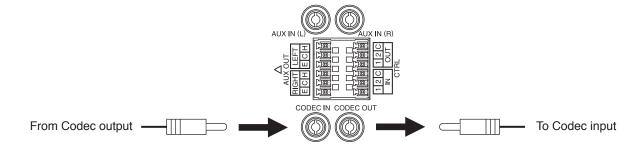
[Codec input (monaural)] RCA pin jack,  $-10 \text{ dB}^*$ ,  $10 \text{ k}\Omega$ , unbalanced
