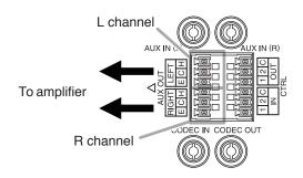
[AUX output] Removable terminal block (6 pins) +4 dB\*, 600  $\Omega$ , balanced (electronically-balanced) \* 0 dB = 0.775 V
