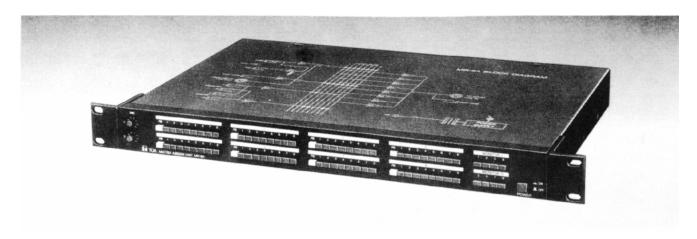
The Toa model MR-8A is a one-rack space Assigner Unit for use with Toa's MR-8T Eight Track Studio Cassette Recorder. The MR-8A adds patch-free channel bouncing, rack and source mixing, and input assignment capabilities to the MR-8T Recorder. With the MR-8A as an interface, connections can be made by means of the switches on its front panel.
