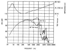
Frequency response is measured in a spherical free-field environment, under 1 watt & 1 meter conditions, with a swept sine wave signal, while the speaker unit is mounted in an 120-liter sealed box. The impedanced magnitude curve is measured while the speaker is suspended in free air, with its cone in the vertical plane.
