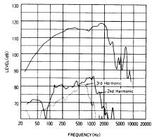
Distortion response is measured with a swept sine wave signal, at 50 watts (-10dB power) & 1 meter, and while the speaker unit is mounted in an 120-liter sealed box
