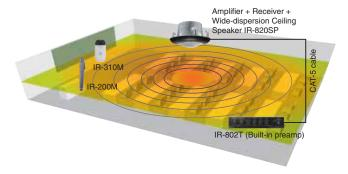
Classroom audio distribution systems (CADS), formerly known as sound field amplification systems, should be used, when appropriate, to achieve clearer speech signals (Larsen & Blair, 2008). With these systems, the signal level is greatly improved since only the voice at the microphone is amplified, not the background noise.
