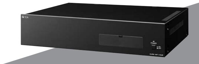
The C-AL80 Alarm Unit serves as the main controller for the alarm requirements of a system by converting alarm signals initiated by externally connected equipment into RS-232C-compatible signal data. In addition to its 32 alarm or remote inputs, the C-AL80 can also be linked to a maximum of 8 other C-AL80 units in master/slave configurations. This provides a total of 256 alarm or remote inputs to be transmitted to the C-RM500 remote controller.
