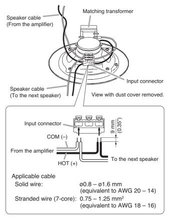
**4-2.** Change the input impedance as needed. The speaker's input is factory-preset to 1.7 k $\Omega$ . When changing the input impedance, detach the black wire connected to the matching transformer, and reinsert it into the desired input tap referring to the table below.
