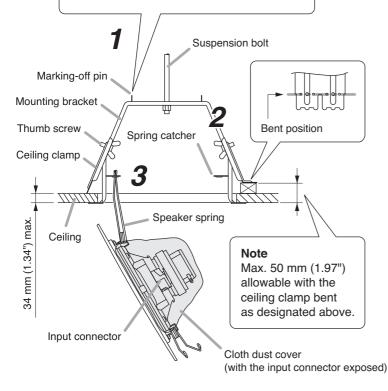
**Step 2.** Place the mounting bracket in the hole and secure it with the thumb screws in the two ceiling clamps.
