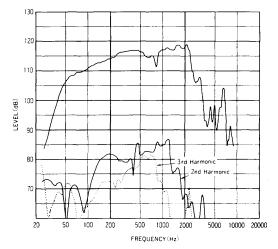
\*Measured at 50 watts (-10dB power), 1 meter reference distance
