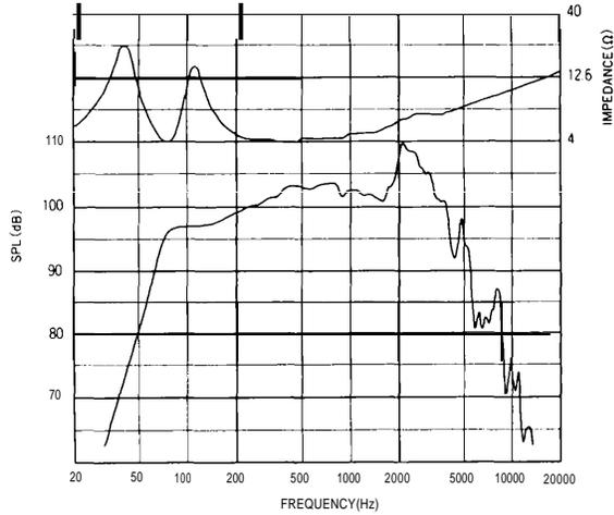
\*Measured in an anechoic environment referenced to 1 watt at 1 meter.
