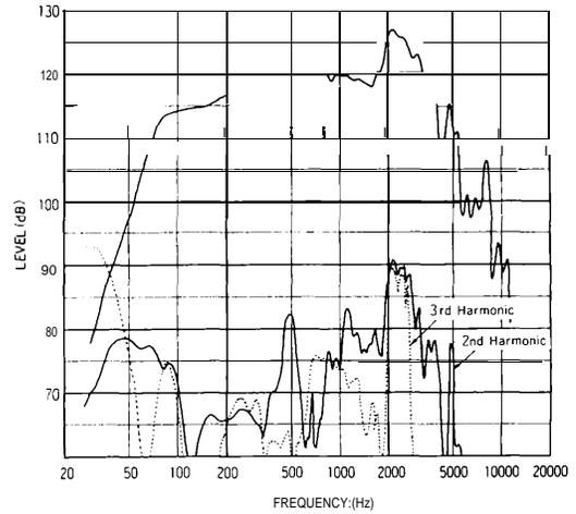
Measured at 60 watts (-10dB power), 1 meter reference distance
