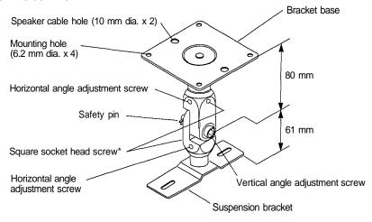
Caution: \* Never loosen two square socket head safety screws for falling-out prevention.
